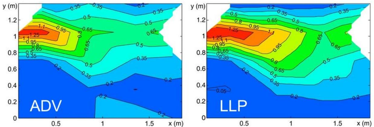
Figure 2. Velocity contours from ADV and LLP measurements at KIT in a scale vertical slot fish pass.
