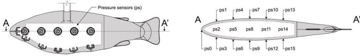
Figure 1. Locations of collocated pressure transducers, all of which are mounted normal to the body surface.
